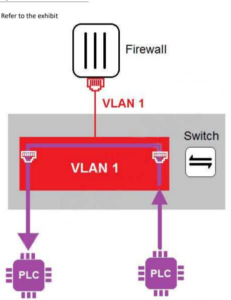
In the topology shown in the exhibit, both PLCs can communicate directly with each other, without going through the firewall.
