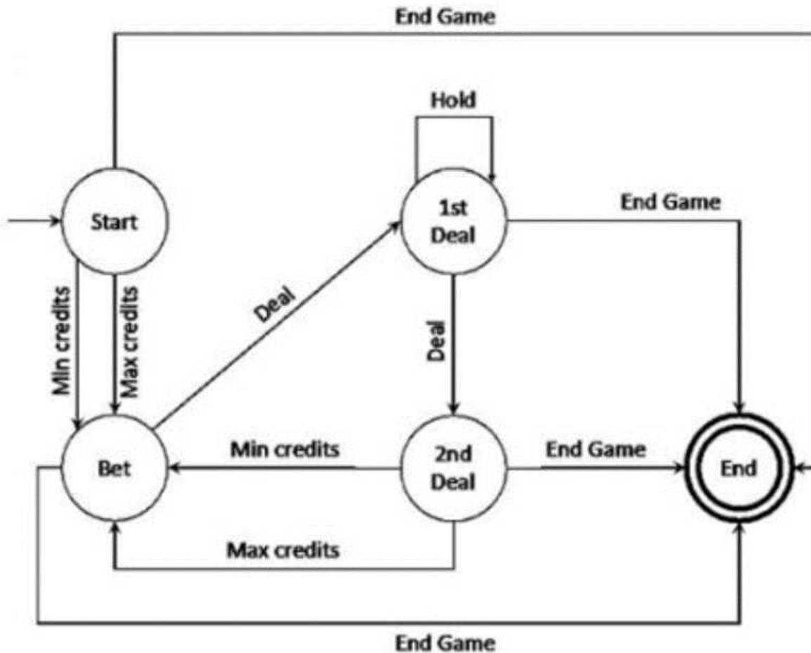
What Is the minimum number of test cases needed to cover every unique sequence of up to 3 states/2 transitions starting In the "Start" state and ending In the "End" state?
